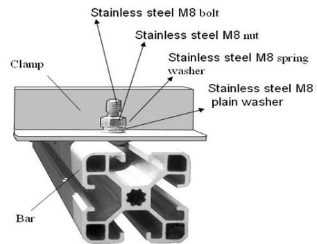
Fig. 8 Schematic diagram of the fringe clamp
